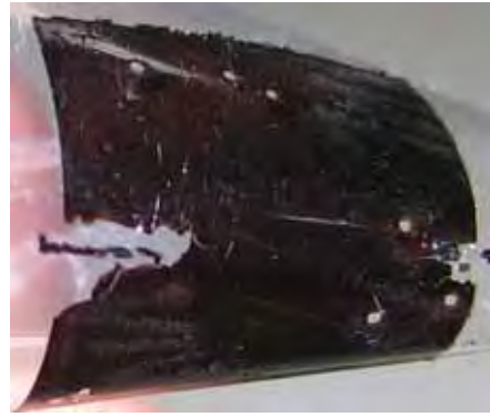
Figure 10: A photo of self-assembly Mn oxide superlattice thin film electrodeposited on the Pt working electrode followed by transferring to an adhesive tape. Large faults seen in the film are due to rough handling of the film before transferred to the tape.
