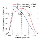
Table -II EQE notable points of QDSL vs QW i-QDSL i-QW EQE EQE High energy photon 0.60 0.4 380 nm Visible photon 1.0 0.7 700 nm Low energy photon 0.7 0.4 900nm
